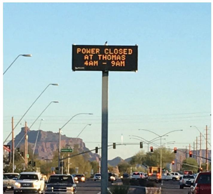
Figure 9. Road Dynamic Message Signs
