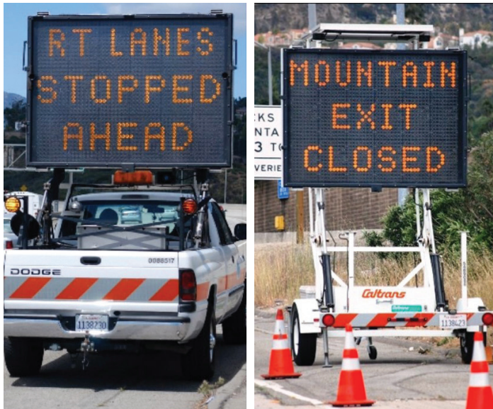
Figure 1. Portable Changeable Message Signs (PCMS). Retrieved from "Changeable Message Sign Guidelines" Caltrans, December 2013
